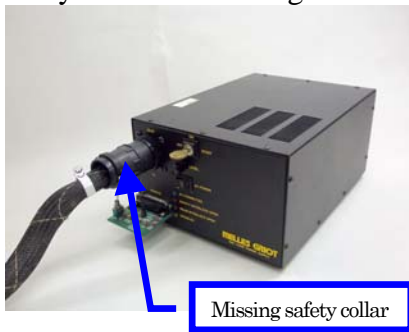
The safety collar is missing at the laser power supply connection.
