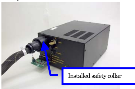
The safety collar is installed at the laser power supply connection.
