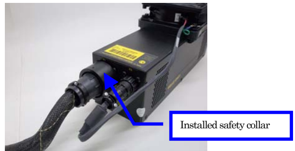
The safety collar is installed at the laser head connection.
